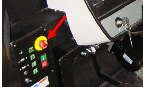
2. To reset, wait 30 seconds, twist the E-Stop button until it pops out, and then restart the simulator.
